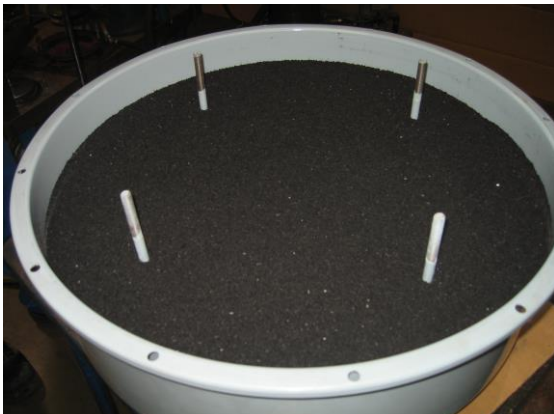
The bottom part of the filter contains carbon, while the top part contains a particle filter.
