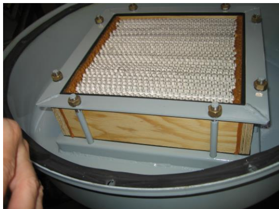
The bottom part of the filter contains carbon, while the top part contains a particle filter.
